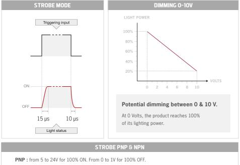
NPN : less than 1V for 100% ON. Above 2V for 100% OFF. Max 20V.
