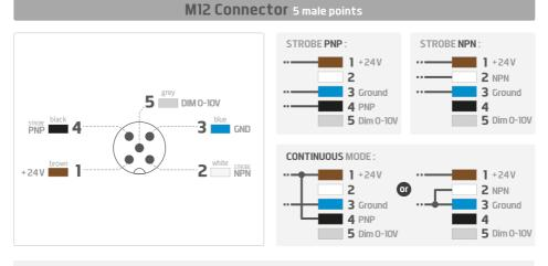
**PNP :** from 5 to 24V for 100% ON. From 0 to 1V for 100% OFF. **NPN :** less than 1V for 100% ON. Above 2V for 100% OFF. Max 20V.
